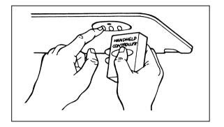
4. Using both hands, push the hand-held transmitter button and the desired button on the HomeLink Transmitter. **Continue to press both buttons through step 5.**
